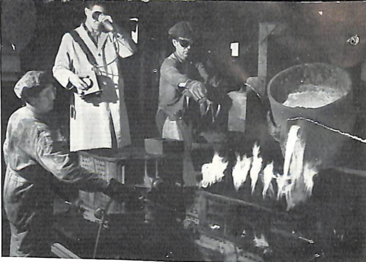
Major castings such as engine blocks, for Australian-made trucks, are poured at Company's Geelong Works. Technician is testing temperature of molten metal with visual pyrometer.
