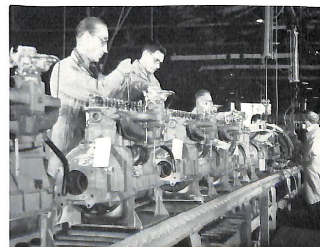
Engines near final stage of assembly when they will be tested and installed in chassis to power new International trucks.
