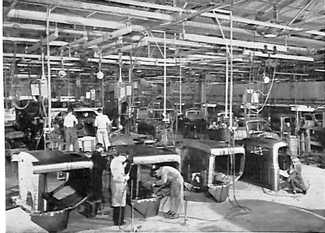
Through complicated jigs and fixtures, pressed sheet metal is transformed into truck cabins and a variety of bodies for Australian-made International trucks.
