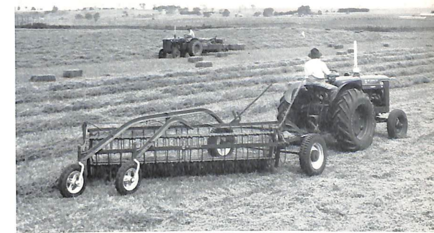
Soon after mowing, hay is raked into neat windrows by McCormick International side delivery rake. Good fluffy windrows assist in even drying of the hay.
