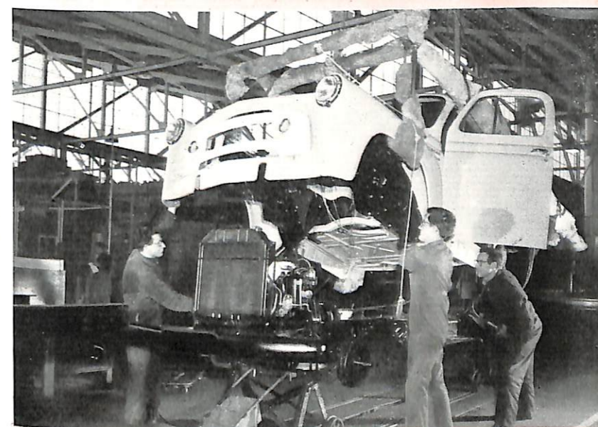
Complete cab assembly is lifted onto chassis, engine and transmission assembly during final stage of production.
