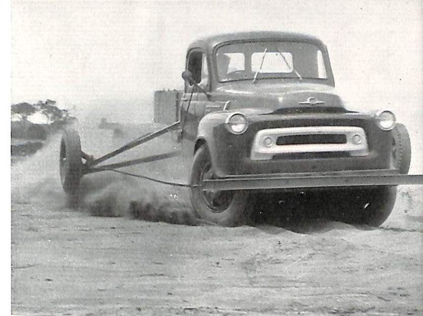
Hard driving and heavy loading test truck stamina in the "Trial by Torture" — an important part of the I.H. engineering research programme.
