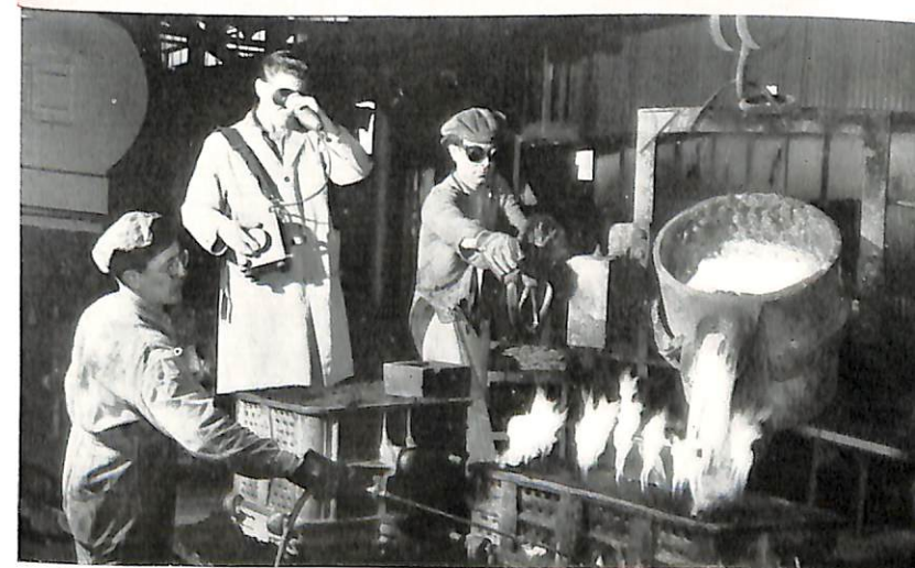
How hot is the molten metal pouring into this engine block mould? Technicians at I.H. Geelong Foundry can "tell by looking" with the visual pyrometer.
