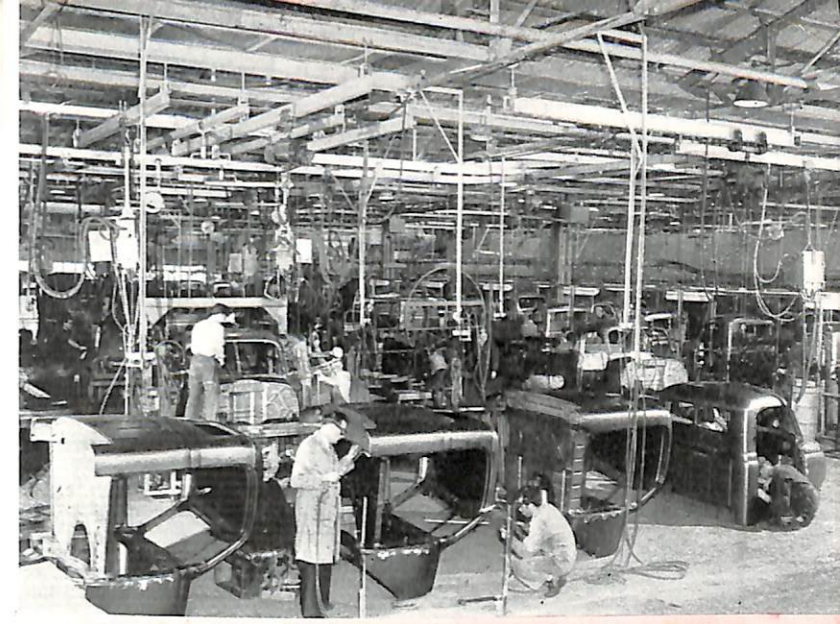
Through complicated jigs and fixtures, sheet metal becomes cabs and utility bodies for the full range of International motor trucks.
