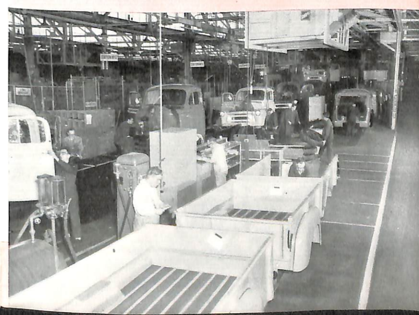
Complete cab assembly is lifted onto chassis, engine and transmission assembly during final stage of production.
