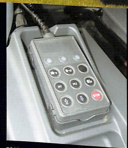
ECAS controls give adjustable selection for the rear suspension to level the deck to dock height
