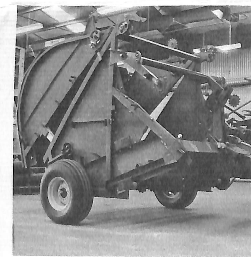
The 850 is taking shape. Still requires pick-up and chains prior to finishing.
