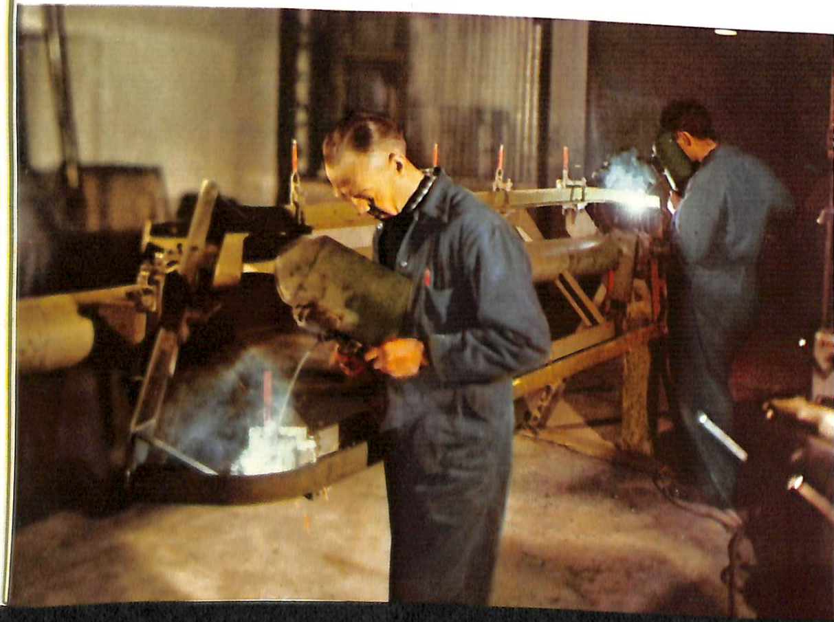
To ensure maximum strength and durability, electric-arc welders at the New Holland plant fabricate the four parts which go to make up the reel basket frame of a "Rolabar" Side Delivery Rake.
