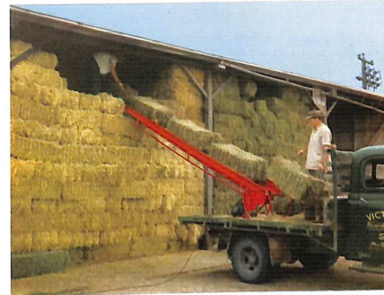
Providing the truly economical answer where baled hay is the only crop to be elevated, this New Holland Bale Booster provides the same time-and-labour-savings as an all-crop elevator, at about half the cost.
