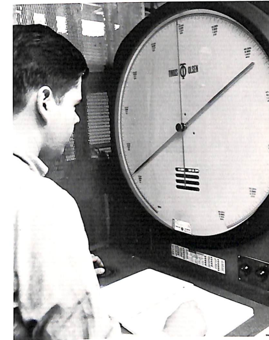
Tensile and compression testing make sure parts and materials used in New Holland machines will stand up under the most rugged field conditions.
