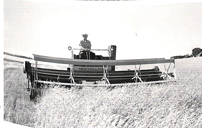
The New Holland self-propelled Speedrower windrower is designed for farmers who need a machine with high capacity to harvest many acres a day during the peak season.
