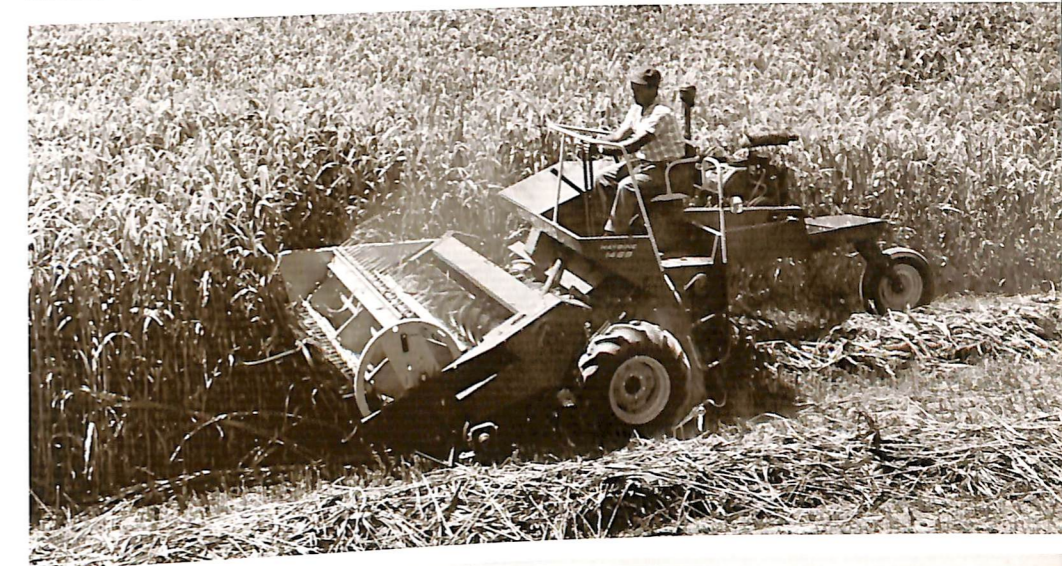
The Haybine mower-conditioner mows, conditions and offers a choice of windrowing or swathing.
