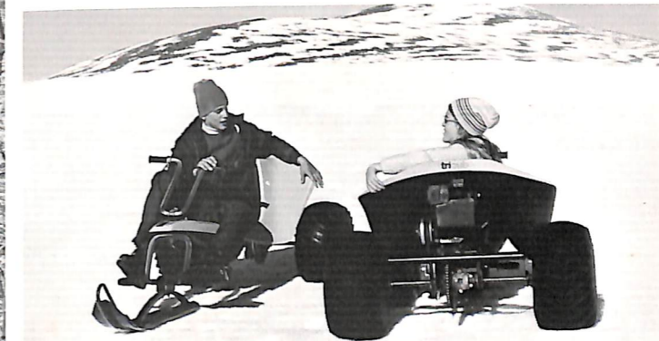
The SPD Tricart sports vehicle combines many of the qualities of the snowmobile, trail bike, dune buggy and all-terrain vehicle in one sporty fiberglass package.
