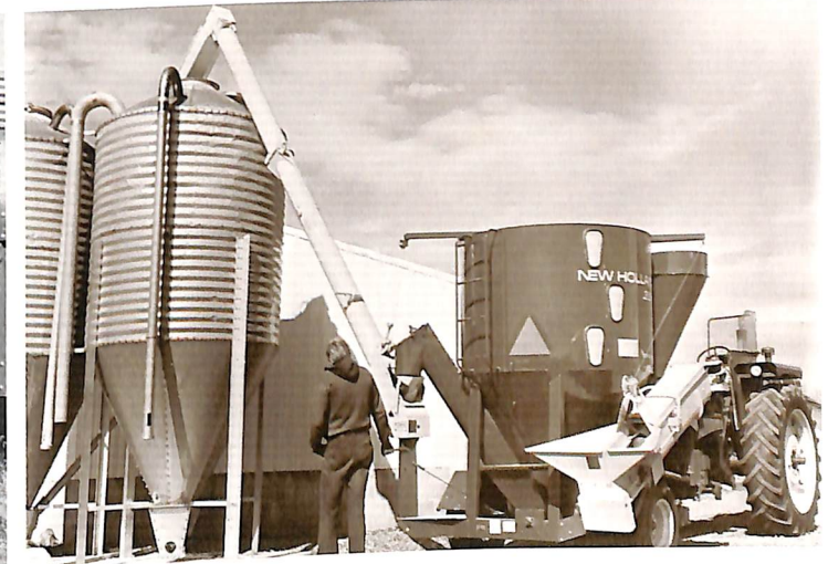
Portable grinder-mixers save farmers time and money. These machines let farmers grind feed more conveniently and economically than buying the service from commercial operators.
