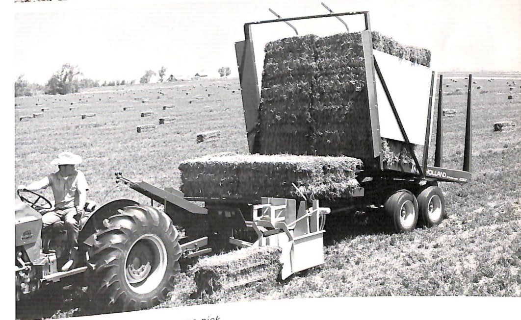
New Holland automatic bale wagons pick up, load, transport and stack bales in one operation.
