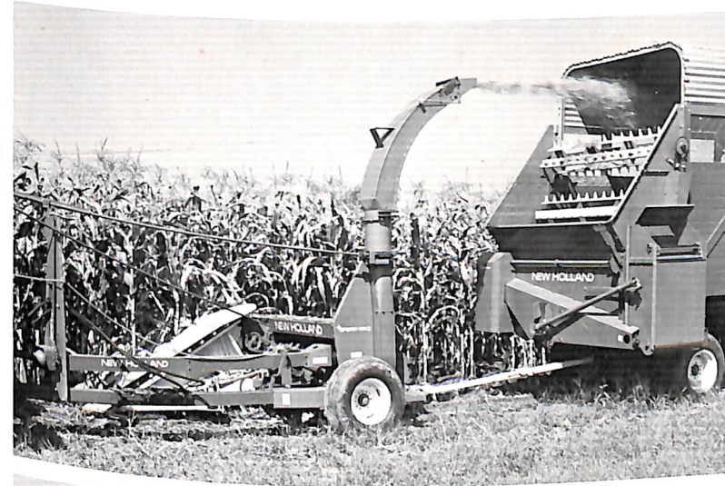
New Holland forage harvesters cut corn as fine as 3/16", and are capable of harvesting 40 tons an hour.
