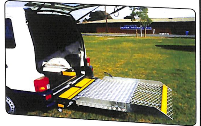
VW Transporter fitted with Wheelchair Lift and Restraint System for Wheelchairs
