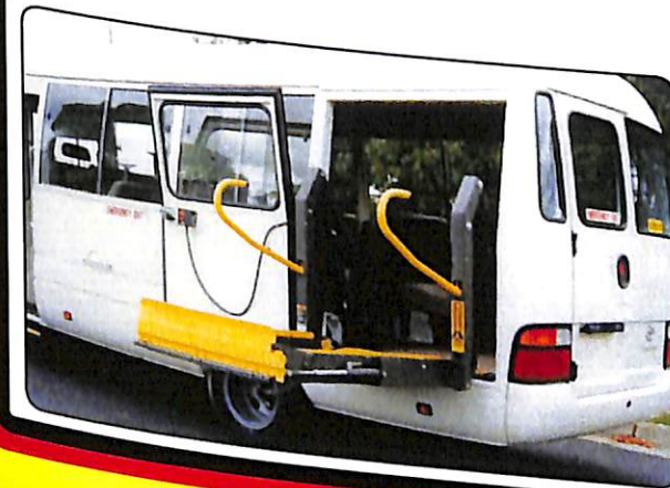
Toyota Coaster Bus fitted with New Side Door and Wheelchair Lift. New Door and Frame Fabricated, Painted and Fitted by Norden
