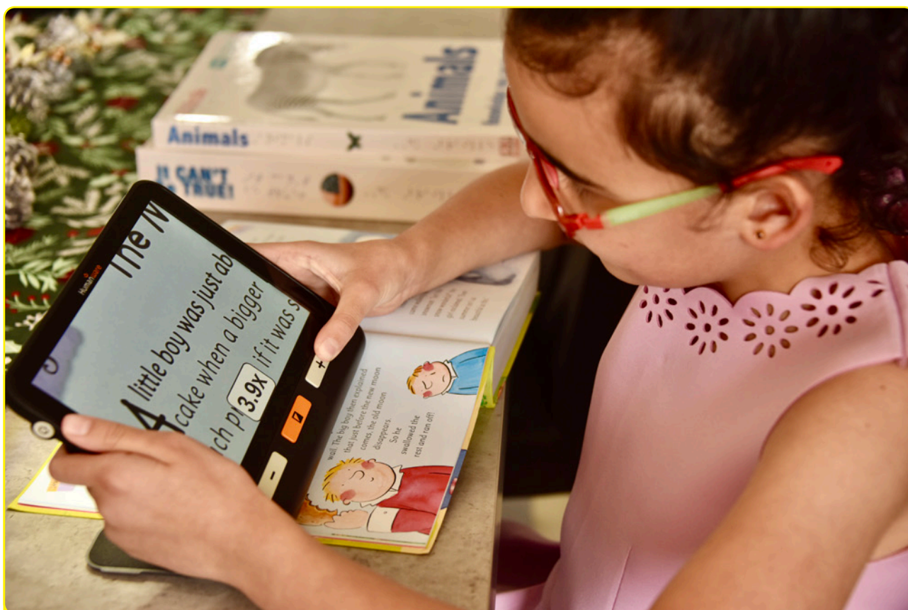
Above: Ten-year-old Haya uses a handheld electronic magnifier that enables her to read a wide array of books and other printed material.
