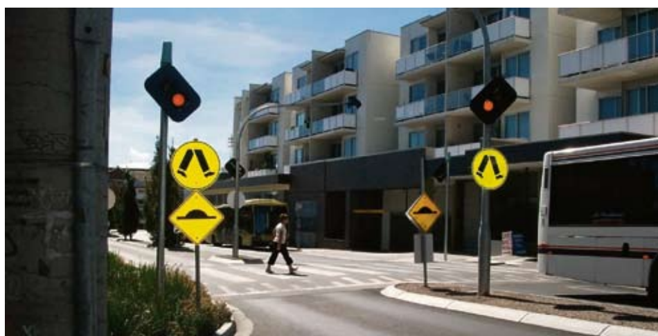
Flashing lights have been installed at the zebra crossing at the Horne Street interchange in Elsternwick. Photo: GECC Traffic Engineering.
