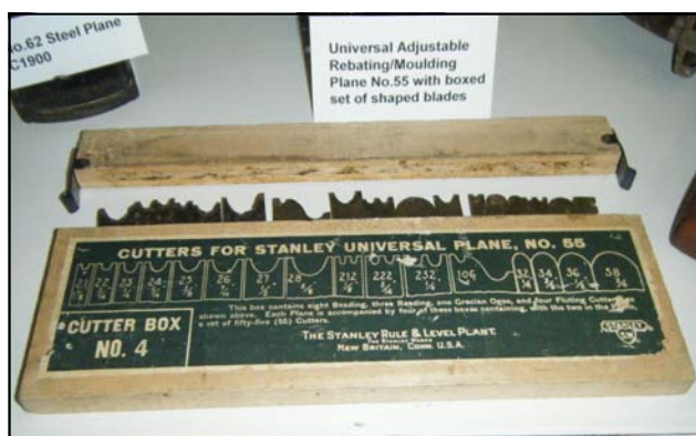
Universal Adjustable Rebating/Moulding Plane No 55 with boxed set of shaped blades
