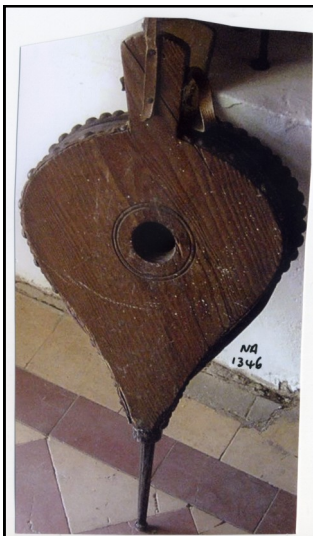
NA1346 A pair of wooden bellows with metal studs, leather inset and metal funnel. The diagram on the right shows the principle on which they worked
