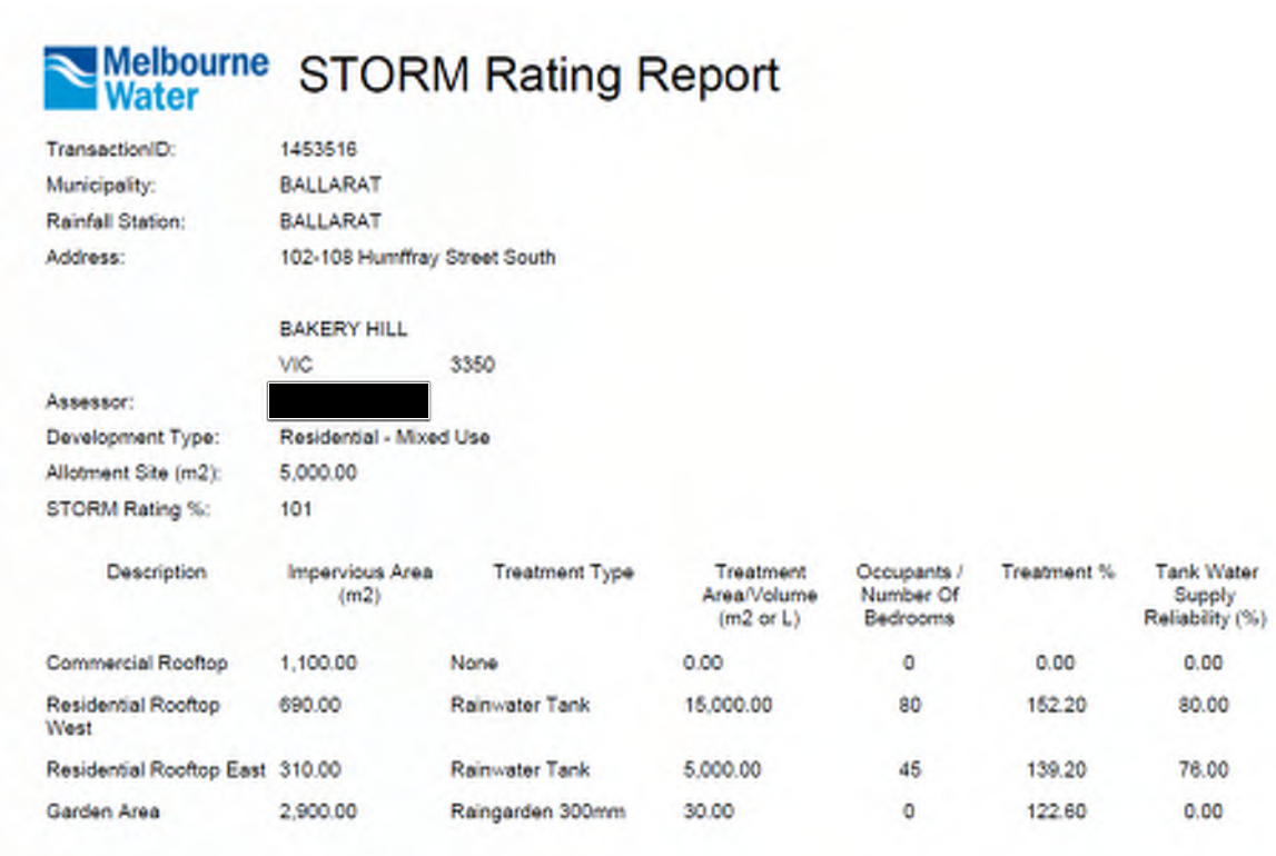
Figure 15: Melbourne Water’s STORM tool showing compliance
