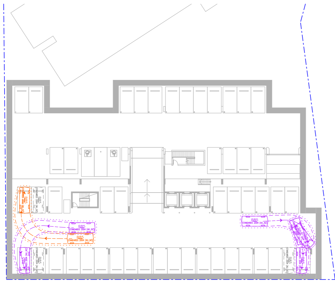
ENTRY MANOEUVRES - - - - - DESIGN VEHICLE SWEEP PATHS SHOWN DASHED ..... 300mm CLEARANCE ENVELOPE SHOWN DOTTED
