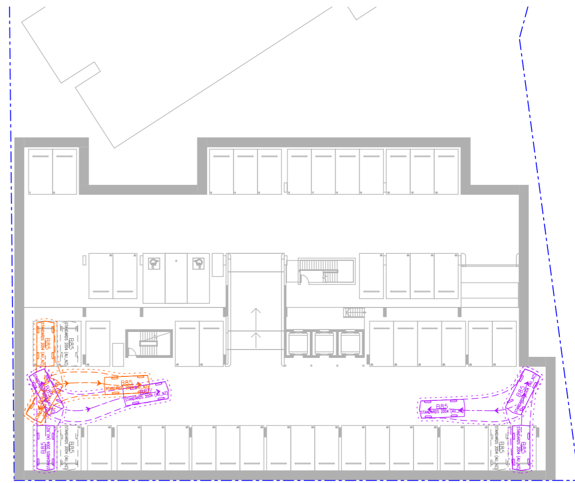
EXIT MANOEUVRES - - - - - DESIGN VEHICLE SWEEP PATHS SHOWN DASHED ..... 300mm CLEARANCE ENVELOPE SHOWN DOTTED
