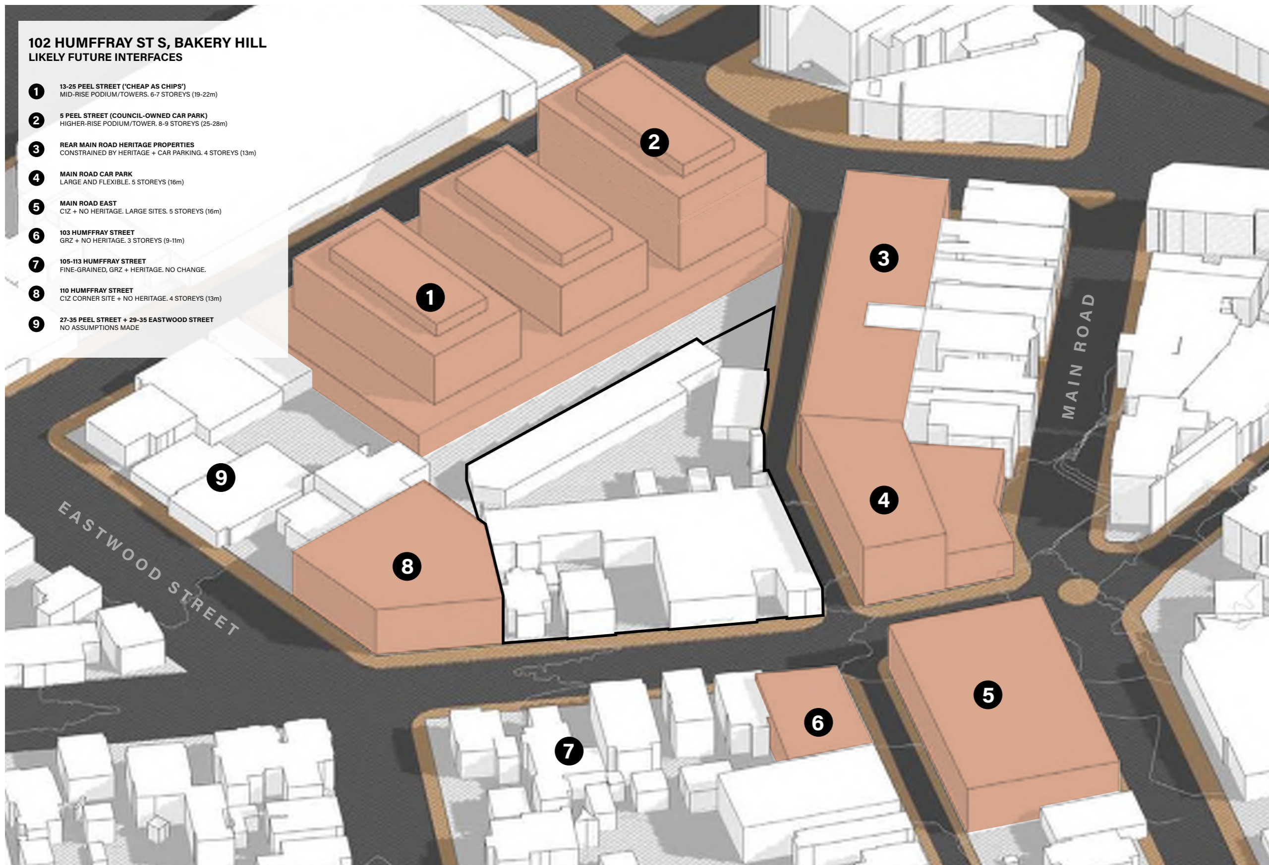
Figure 42 - Equitable development diagram showing likely future development scenarios on adjoining and opposing properties
