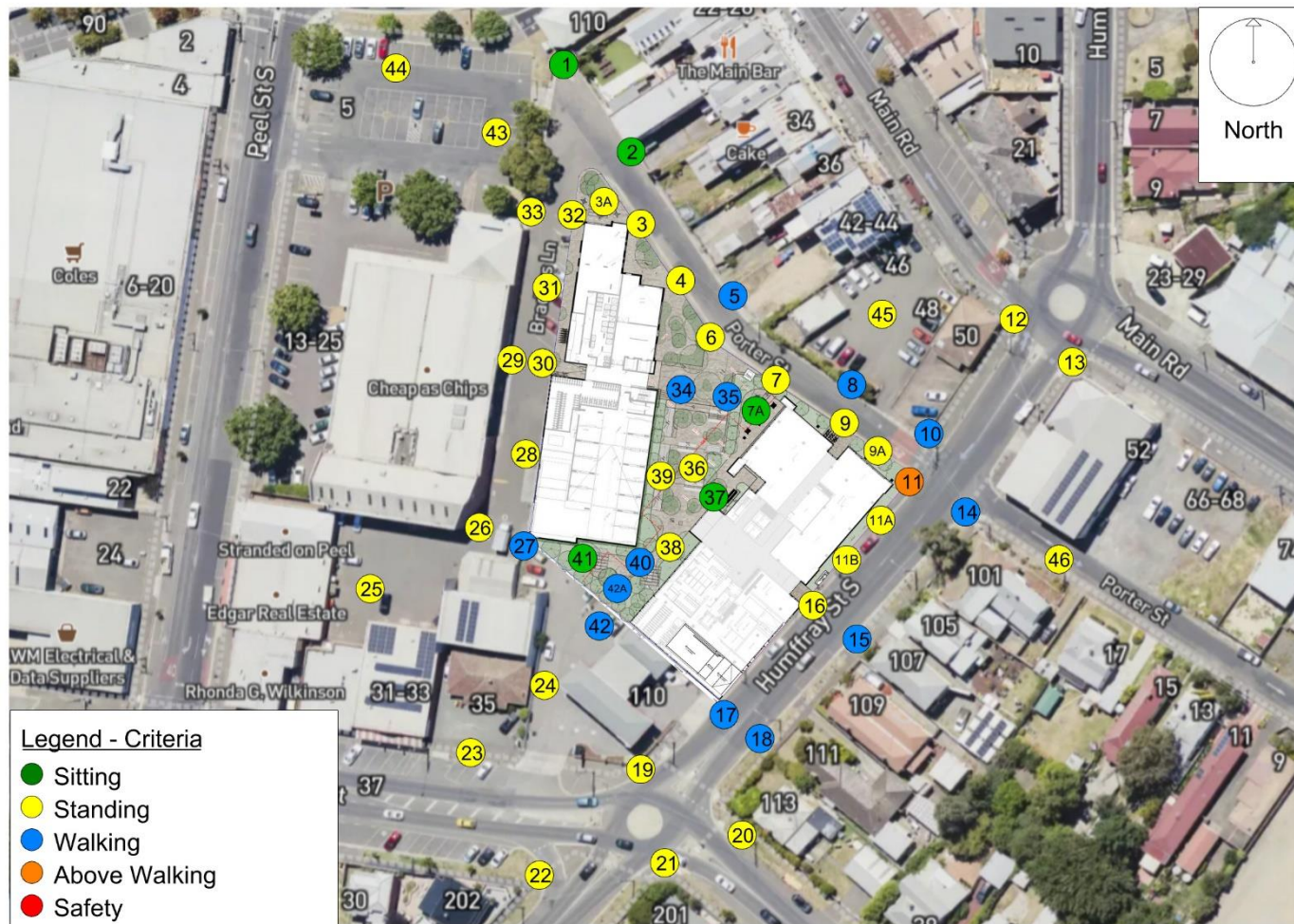
Figure 6b - Summary of wind conditions at Ground Level Test Locations around the 102-108 Humffray Street Development for the Proposed Configuration (no landscaping) for 360° of wind direction
