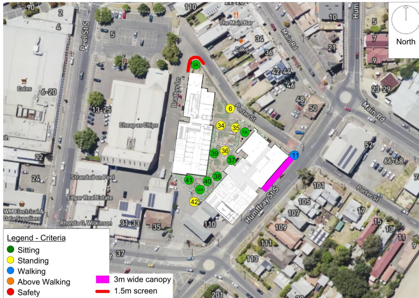
Figure 6c - Summary of wind conditions at selected Ground Level Test Locations around the 102-108 Humffray Street Development for the Proposed Configuration with Plaza landscaping and mitigation strategies.
