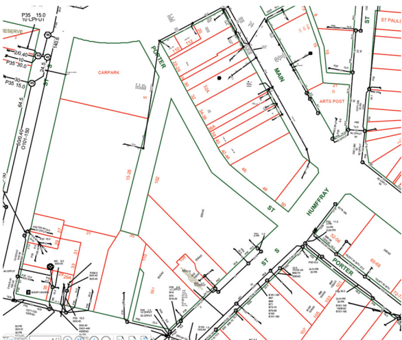
Figure 10 Existing Telstra Infrastructure DBYD©
