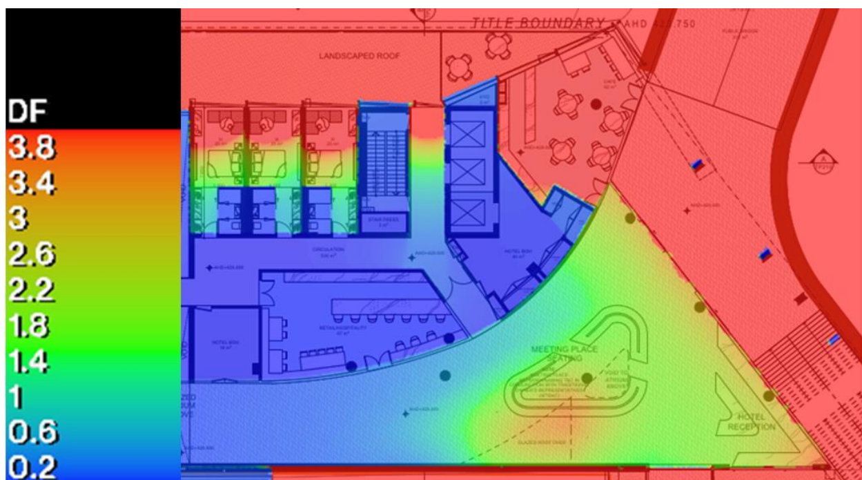
Upper Ground Zone 1 Daylight Factor Contour Plot
