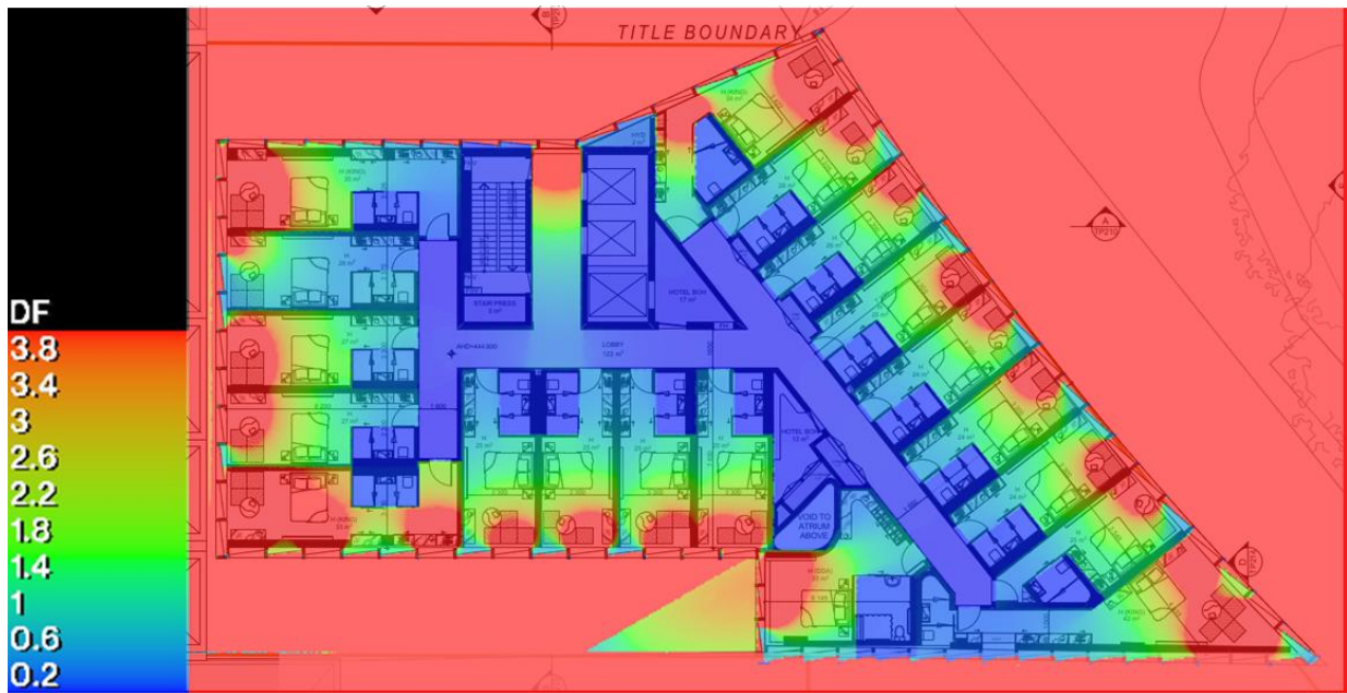
Level 6 Zone 1 Daylight Factor Contour Plot
