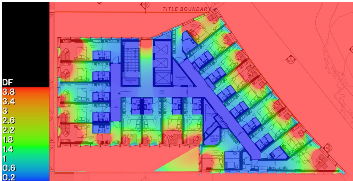
Level 5 Zone 1 Daylight Factor Contour Plot
