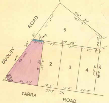
MEASUREMENTS ARE IN FEET AND INCHES DERIVED FROM VOL.6714 FOL.624 29.4.'68.
