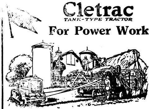
24 B.H.P. at the Pulley, driven direct off crankshaft. Power available for every class of work. The "Cletrac" drives to and does—the job, replacing 8 horses and 20 H.P. Stationary Engine. Runs on Kerosene.
