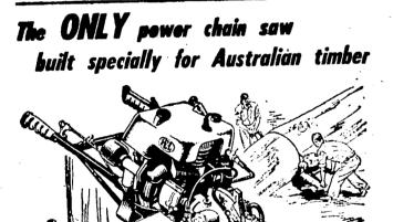
Whether you're felling trees for the mill or on general timber construction work, you'll find this efficient w a tireless worker. It goes anywhere a hand cross-cut goes and does a cleaner job in a fraction of the time. In wide use by timber-getters here and overseas, it is efficient in both hard and soft woods-cuts at any angle; simple te operate and maintain.
