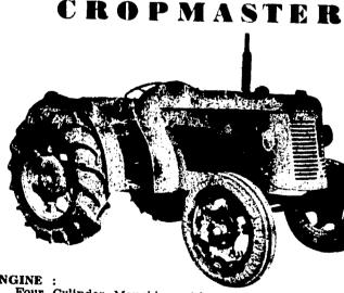
Four Cylinder Monobloc with Wet Cylinder Interchangeable Sleeves. Detachable Head carries all Valve Gear. Bore, 31 in.; Stroke, 4 in.; 25/35 b.h.p. all range governor operating at all speeds from 600 to 2000 r.p.m. Many improvements and advantages, such as hydraulic lift, 2-speed take-off, belt pulley and additional rear clutch have been made. This modern tractor replaces an 8 horse team.
