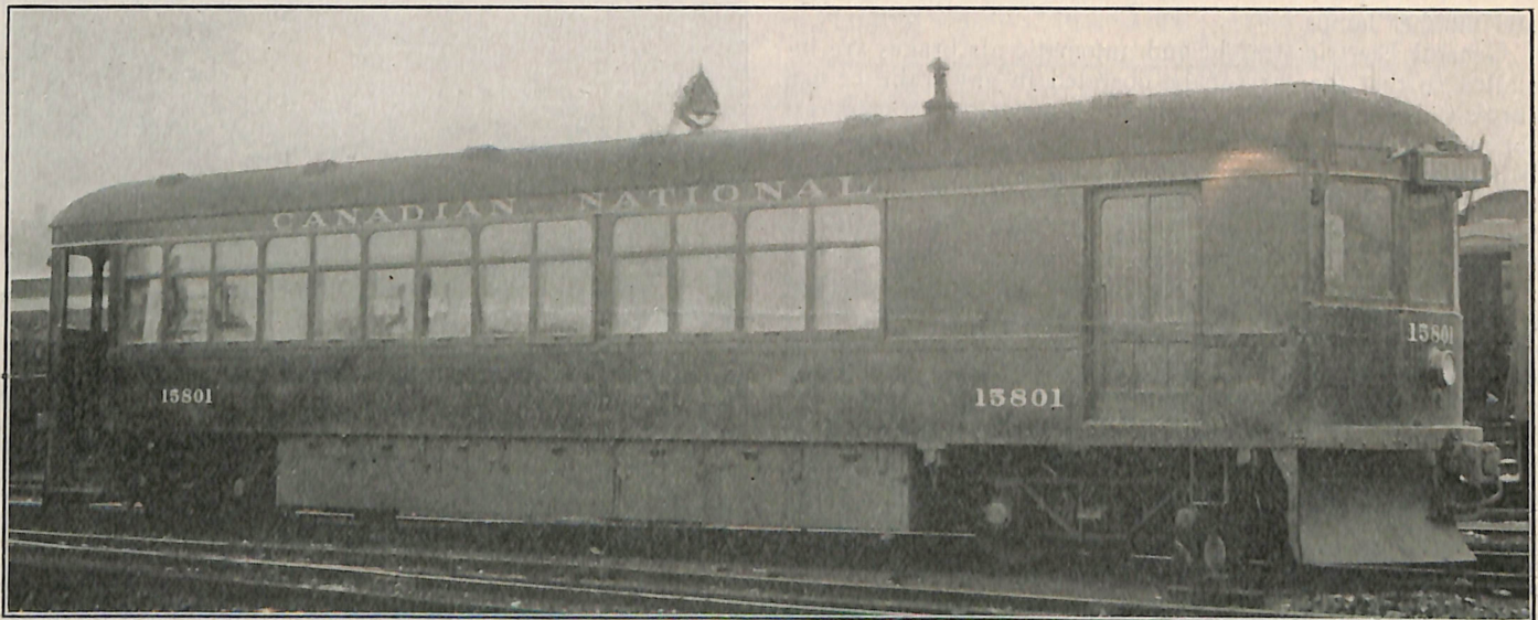
Car No. 15801 is Equipped with Four 25 hp. General Electric Motors, 2 Type K-36 Controllers, G. E. Straight and Automatic Air Brakes and Complete with Double Flooring, Storm Windows and Extra Battery Box Lining, Weighs 33 Tons
