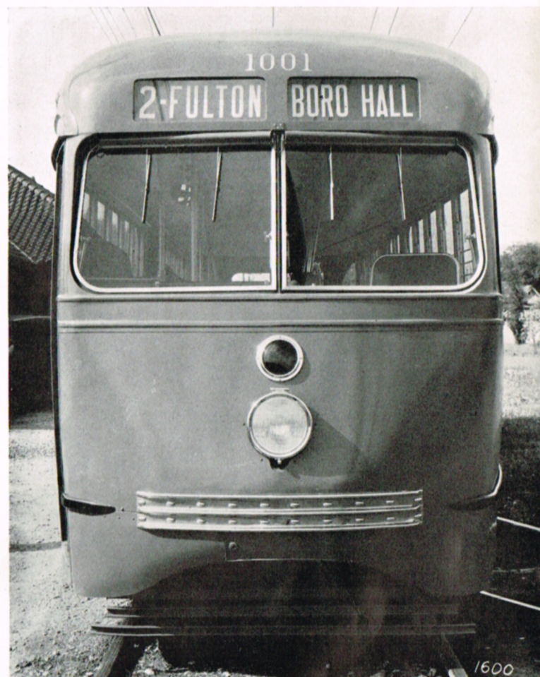
● Front View of P. C. C. Car, showing Windshield-Type Vestibule Windows, Destination Signs, Etc.
