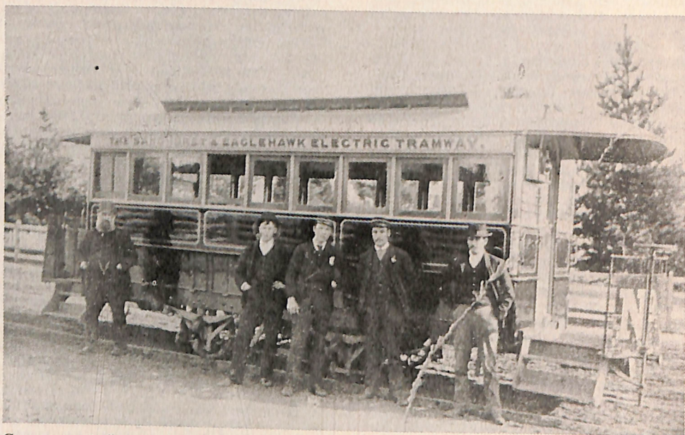
Company staff pose for the only photograph known to exist of the battery tram era. Above the truck with its railway type suspension, the hinged side panels for access to the batteries are clearly visible.
