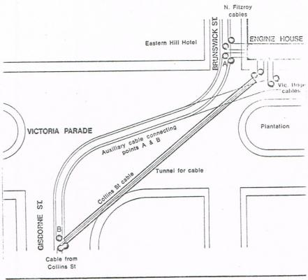
Victoria Parade Junction: the Collins St cable by-passes the curve which is served by an auxiliary cable
