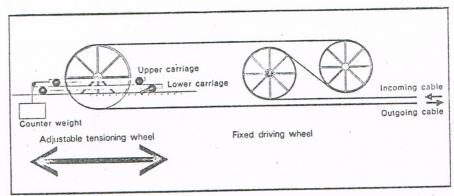
Tension gear: upper and lower carriages (left) are movable to take up cable slack
