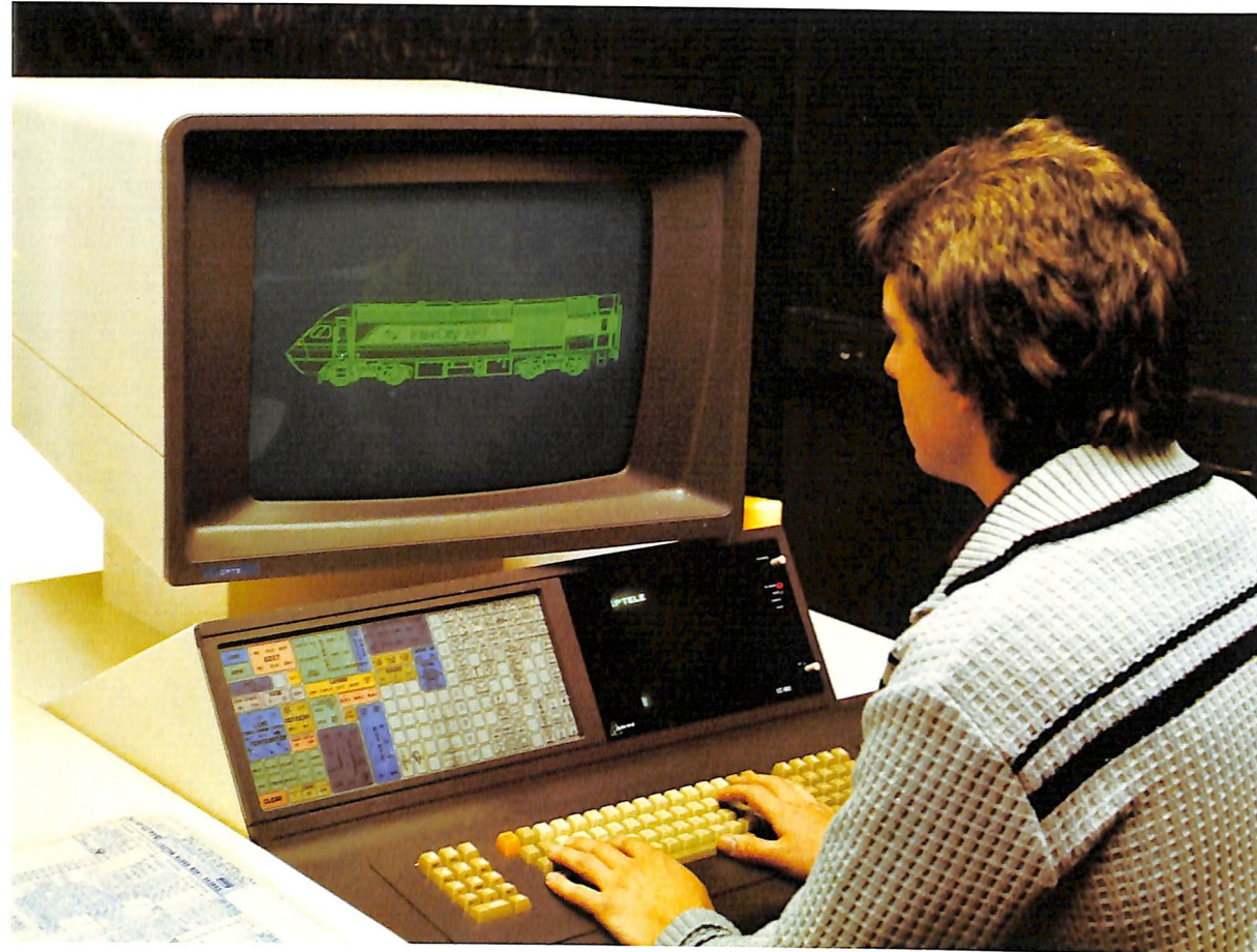
Computer aided design terminals (above and right). CAD allows pre-testing of designs and componentry and permits easy assessment of any modifications. It was widely used in the design of both the 'A' class and the Articulated trams.
