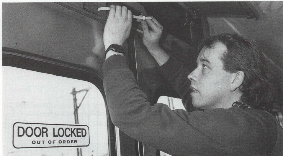
The cable ties keep around three more trains in service during the evening peak. Equipment Examiner, Stuart MacDonald, shows us how it's done
