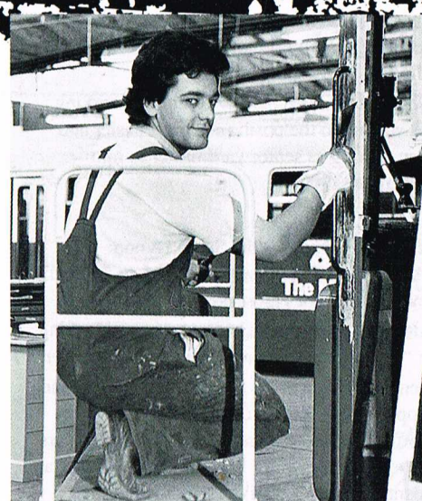
Vehicle Painter, John Vlahakis, burns off 50 years of paint from a vintage tram to restore it to original
