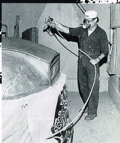
Vehicle Painter, Frank D'Amico, paints the roof of a W class tram in the spray paint booth which controls fumes
