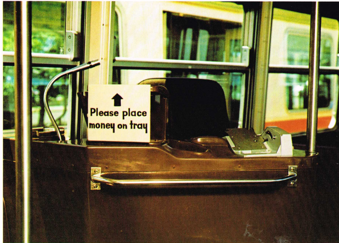
Conductors (if required) equipped with automatic change issuing machine minimise boarding time.
