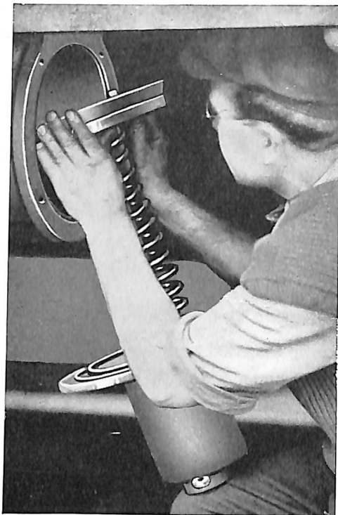
Fig. 22. Showing Initial Step in Fitting Piston Packing Cup into the Brake Cylinder
