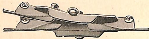
OVERHEAD FROG FOR CENTRE-RUNNING TROLLEY.
