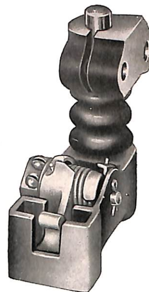
Fig. 13. Brush-holder for Type CP-27 Air Compressor
