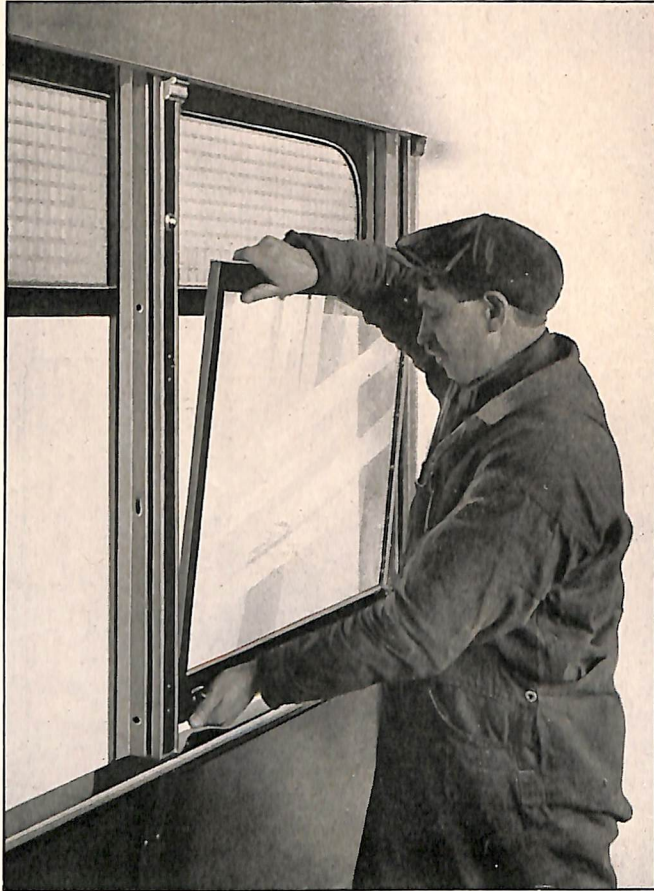
The illustration shows a window sash being removed from its Renitent Post casings by an ordinary workman, without the use of tools. The sash cannot be disturbed from its casing by the casual pressure exerted by a passenger raising or lowering it, but, on the other hand, to remove it does not require super-human strength or painful wrenching
