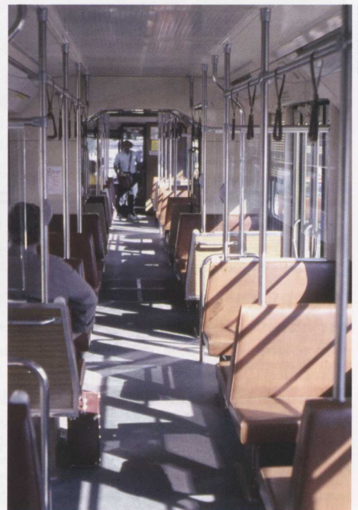
This shot of 2001 at Preston workshops taken in May 1984 shows the steps lowered at the front door, and folded up at the other doors.
