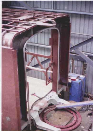
The rear end of one of the articulated trams showing the outriggers that support the body on the centre bogie's slewing ring.
