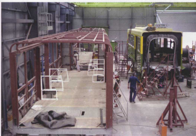
The prototype articulated trams in various stages of construction at Comeng Dandenong.
