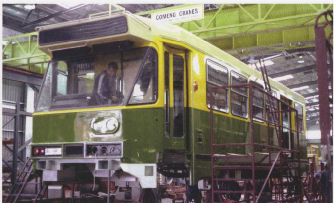
One half of a B-class tram being fitted out.
