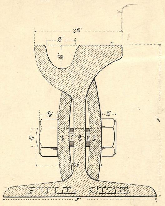
SECTION OF 57LE BESSEMENSTEEL PAILS WITH FISH PLATES ETC
