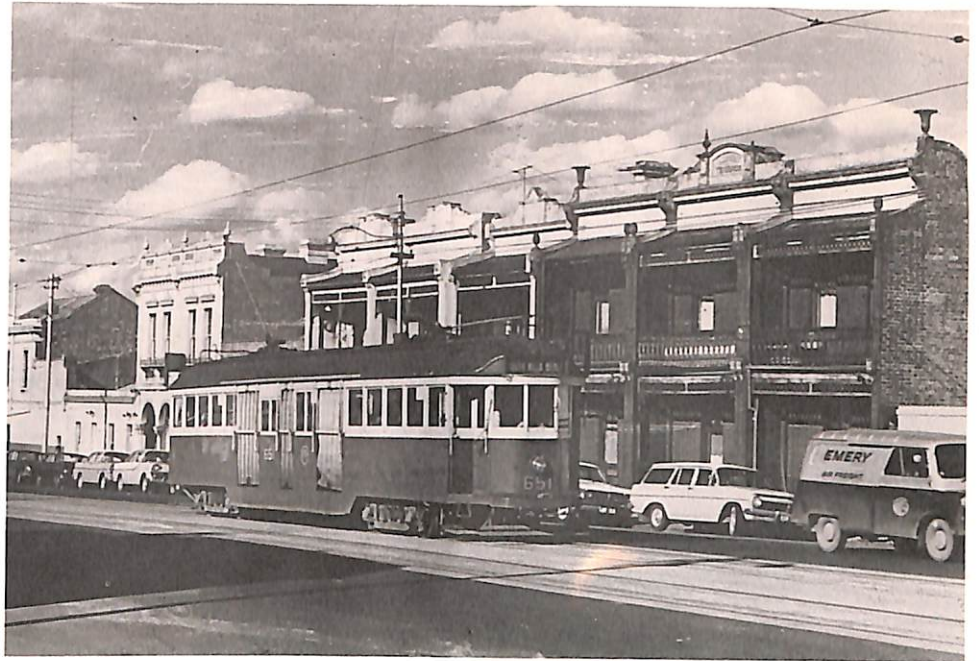
One of the M&MTB's typical standard W-2 class cars in its Hawthorn green and cream livery trundles past the ubiquitous inner suburban terrace while bound for South Melbourne Beach, its No. 1 MCB trucks highly visible in this view.
