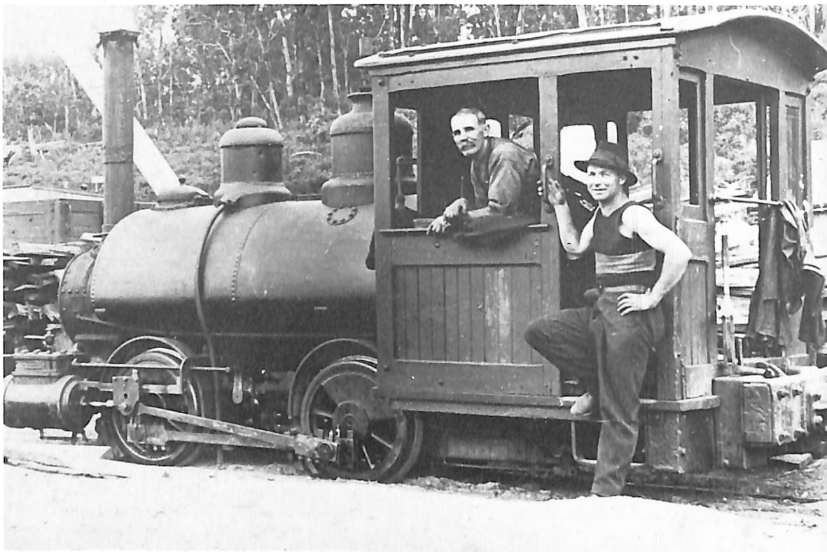
Loch Valley Timber Co Baldwin engine photographed in VR Noojee station yard circa 1920. This is one of the two Baldwins bought from the Sorrento Tramway Co in 1920 (B/Nos 9086 or 12007) both of which had been reboilered, as indicated by the rectangular plate on the smokebox.
