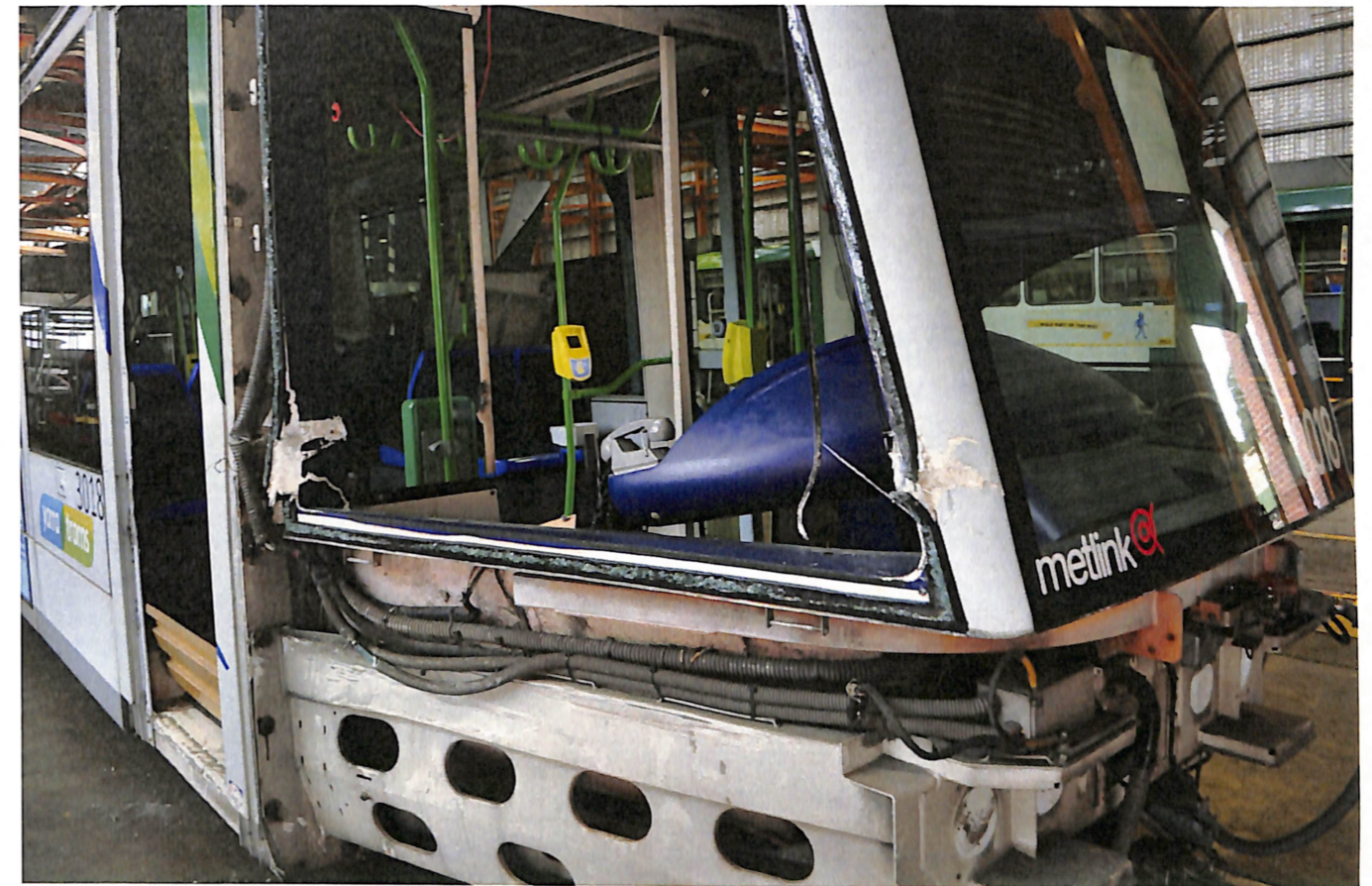
Damage from a major accident after a truck hit tram 3018. The design of a Citadis tram means that the entire driver's cabin has to be dismantled for the repair work to be done. The cost of the job could be over a hundred thousand dollars.
