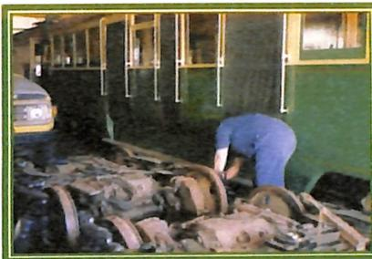
*Kym Smith making final adjustments and lubricating the trucks for L 103 prior to their reinstallation.
