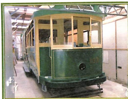
Other site projects took precedence during 2007, but finishing works continued such as the reinstallation of seating, fitting of handrails and hand straps, polishing of brass components, and refitting of windows and doors.
