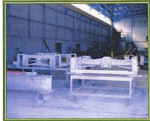
*The truck frames from L 103 after being sandblasted and primed.
