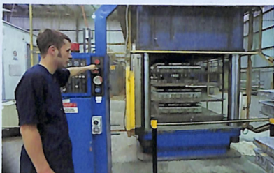
Light-rail door systems. Assembling the control mechanism (top), pressing the panels (above), and testing the system to the limit (below)—this door has been opened and closed 3,000,000 times and it's still going strong.
