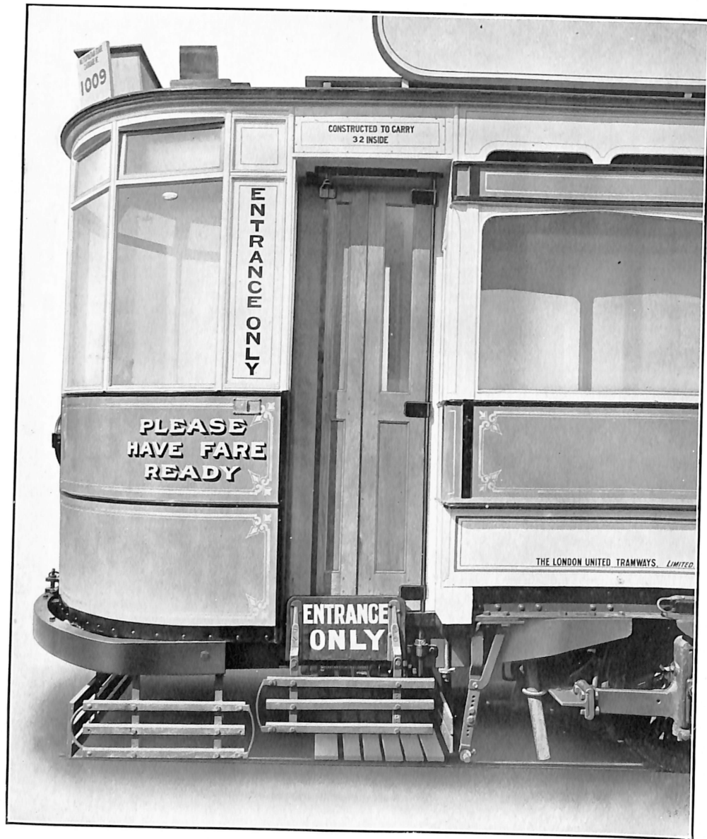
Fig. 2. Outside view of "One-Man" Tramcar, equipped with Automatic Pneumatic Door Control System, showing Entrance Door and Step in closed position.
