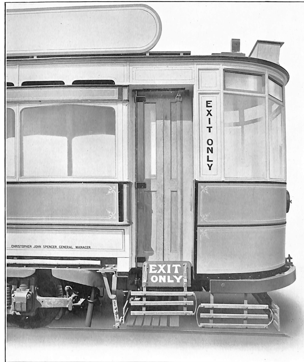
Fig. 1. Outside view of Treadle Plate Controlled Rear Exit Door and Folding Step (closed).
