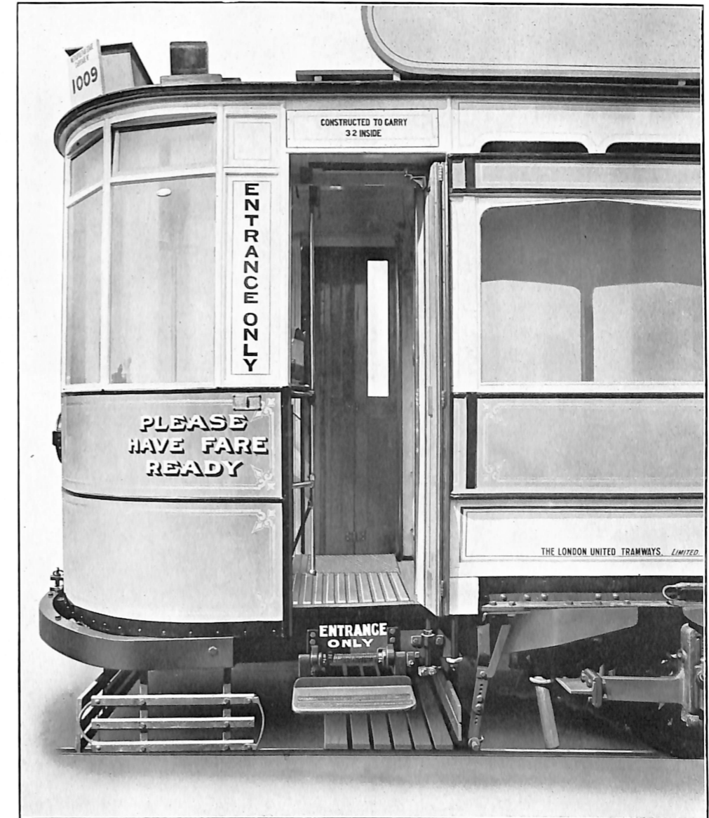
Fig. 2. Outside View of Single Folding Door and Folding Step Gear (open position).
