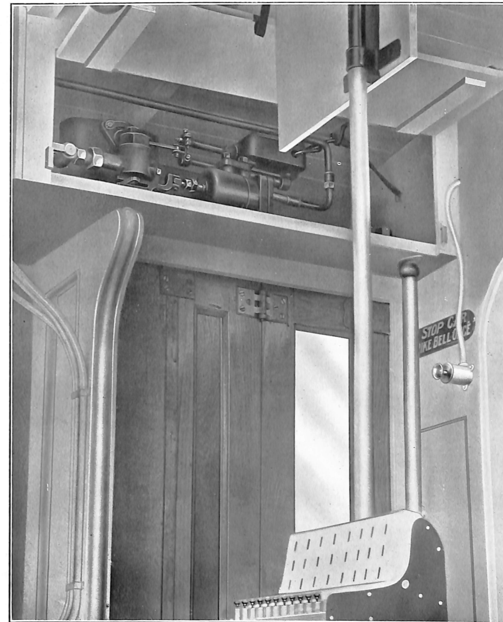
Fig. 2. Interior view showing Type "E" Folding Door Engine mounted in header box over Single Folding Rear Exit Door. (Note the change-giving machine in foreground.)
