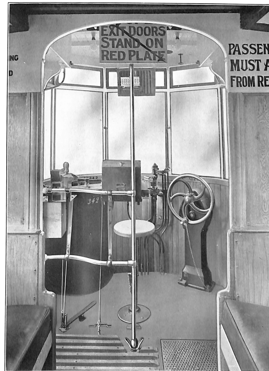
Fig. 1. Interior View of Driver's Position on "One-Man Car," showing Treadle Plate.
