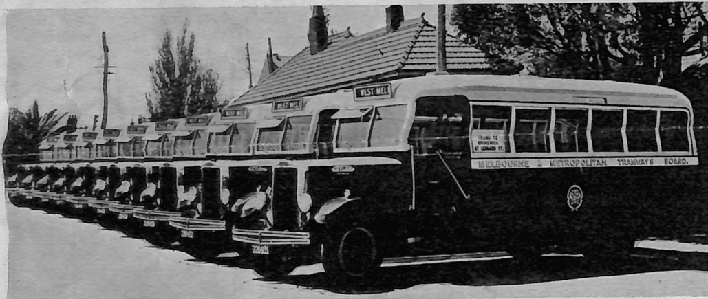
Leyland Cub buses in the service of the Melbourne and Metropolitan Tramways Board, Australia, during cable tramway electrification. Leyland diesel units are now being acquired for tramway replacement.
