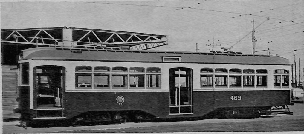
Car designed for tourist service, with one- or two-man operation. Weighing 16½ tons, it has four 40-h.p. motors and an overall length of 45 ft. 6 in.
