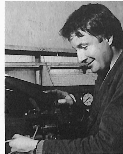
Mike Barker tests a bus brake valve after repairs have been completed. The testing equipment was designed and built by the employees at the Clock Shop.
