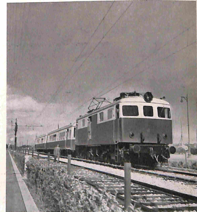
The recently electrified railway between Estoril and Lisbon (Portugal) operates with G.E.C.-equipped electric locomotives and motor-driven coaches.
