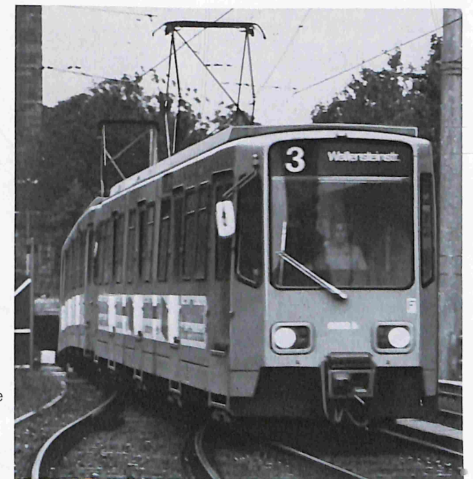
The first articulated tramcar equipped with chopper control for the Stadtwerke Graz (Austria) 1972
