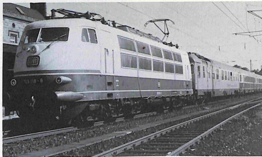
High-speed express locomotive 103 118-6 of the Deutsche Bundesbahn for 250 km/h 1969
