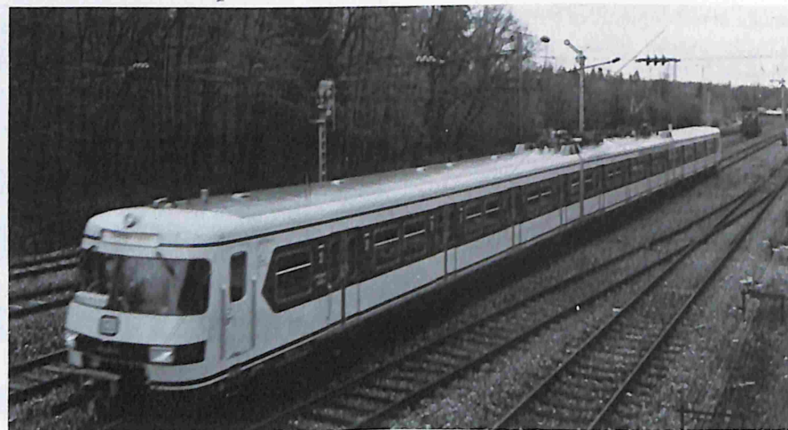
The new thyristor-controlled articulated heavy rail transit car unit class ET 420 of the Deutsche Bundesbahn 1972
