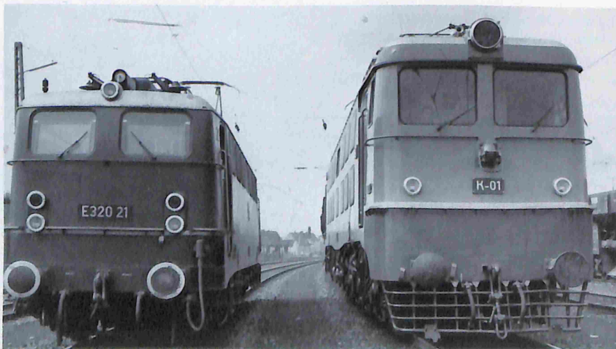
Class E 320 21 two-frequency locomotive (left) and the first class K locomotive, delivered to the USSR 1959
