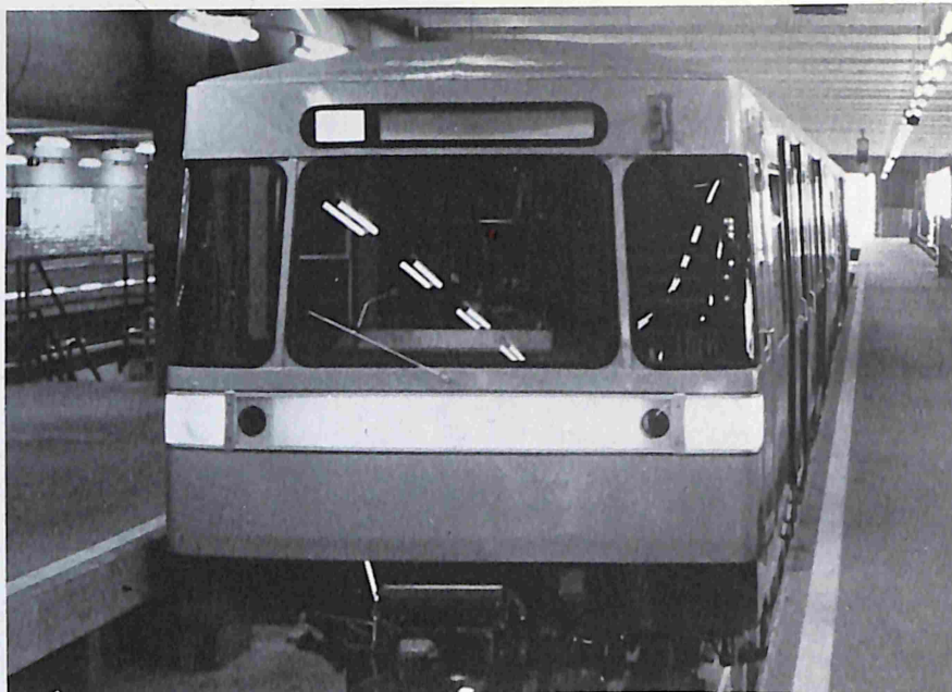
Double motor-car unit with alternating current drive for the City of Vienna 1977
