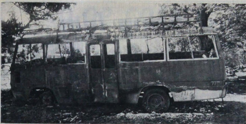
Dripping remains of an aluminium boat on the roof of a burnt-out bus.
